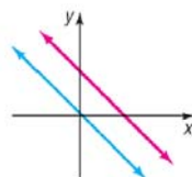
(b) Parallel lines; system has no solution
